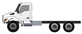
Recommended payload center of gravity to achieve specified ground loads; measured from centerline of drive axles: 31 in. from the centerline of the drive axle(s).
