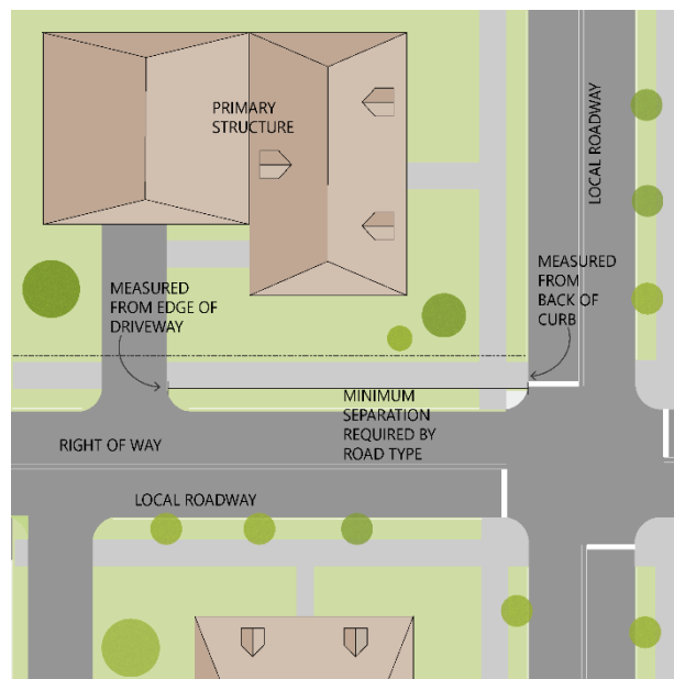
Example of Driveway Separation
