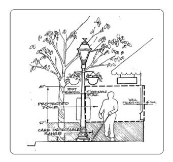
Figure 1 Protruding Objects Requirements
