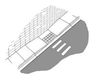
A parallel curb ramp consists of two ramps joined in the middle by a landing that is level with the roadway. Parallel curb ramps run parallel to the curb and usually take up the whole width of the sidewalk.
