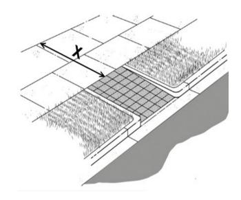
Space is needed at the top and bottom of ramps so people using wheelchairs can align with the running slope and maneuver from ramps, including when making turns (which is difficult on sloped surfaces). ADAAG 4.7.8 defines obstructions in the pedestrian environment as objects that limit the vertical passage space, protrude into the circulation route or reduce the clearance width of the curb ramps.
