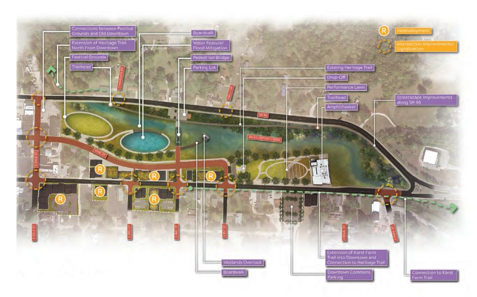
Plan view of a proposed stormwater park
